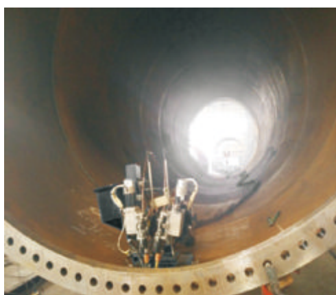
Section flange welding
